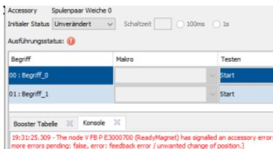
If a drive does not switch correctly, a consumer is no longer connected or an error is detected - then a red exclamation mark is displayed and an error is reported in the console.
