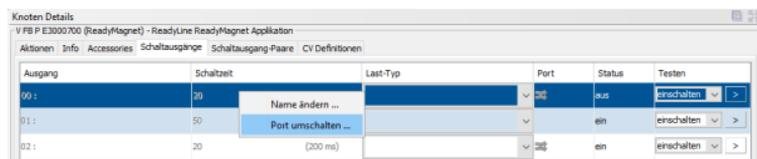
In the factory default setting, the module is configured for 4 switching output pairs with a switching time of 200ms and without limit switch. In the window SwitchPair ports these settings can be changed and adapted to your requirements.
