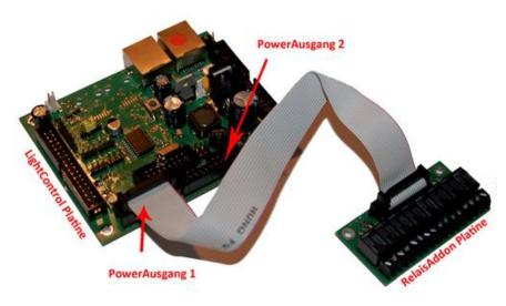
The add-on relay board can be connected to one of the two power outputs at the Lightcontrol PCB. Connection is made with a 16-pin ribbon cable.
